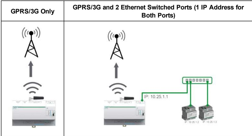
GPRS/3G access can be added to the Com'X 510 by installing a modem under the cover.
