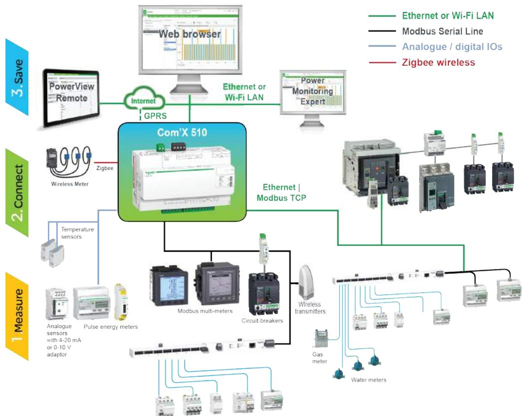
From a simple metering installation with one device to large metering systems, the Com'X 510 collects data from any Modbus TCP/Modbus serial line gateways, pulse meters, actuators, and analog sensors.
