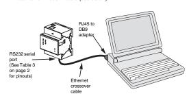
NOTE: The RJ45 to DB9 adapter and the Ethernet crossover cable are included in the TCSEAK0100 configuration kit (sold separately)
