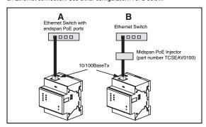
NOTE: Use a PoE injector that fully complies with the IEEE 802.3af standard for active midspan devices, such as the TCSEAV0100 from Schneider Electric.
